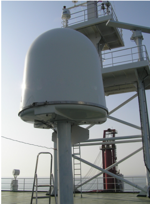
A typical marine VSAT system
